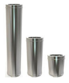
1000MM CONNECTING STARTER LENGTH Code:10-\*\*\*-021 Working length 957mm – with integrated adaptor. This length allows the Clearline Single Skin to socket up into the section by 325mm, then back down to connect to the stove. This part allows the stove to be removed later without dismantling the chimney system, so as to comply with building regulations.
