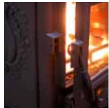
5. After 5-10 minutes the chimney draft should be established, at this point close the fire door. If all the necessary conditions are met, a nice layer of embers will start to accumulate after another 15 - 20 minutes.
