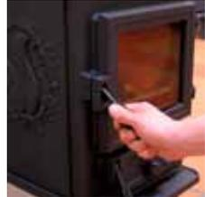
8. When the secondary air supply is opened all the way and the door is closed, the new fuel will ignite in a few minutes.
