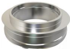
INSULATION COVER PLATE Used to close off a flue system to cover any exposed insulation material. Can be used when using a generic cowl or when no rain cap is required.
