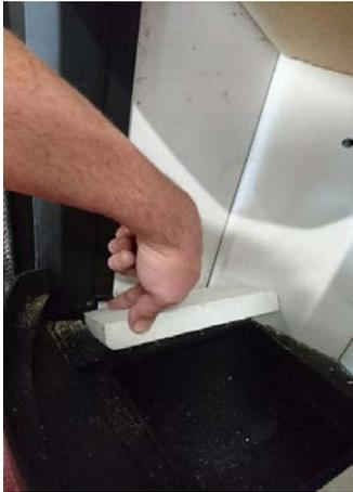
*Remove grate and base fire bricks.*
