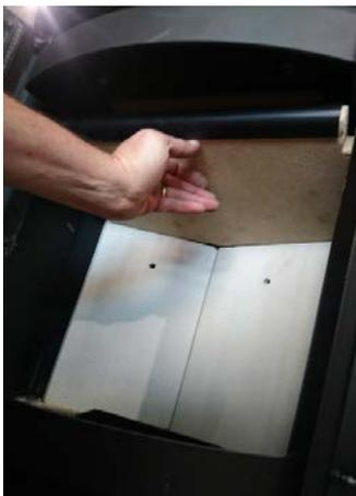
*Now lower the throat plate baffle to remove.*
