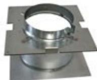
A **ceiling support** is a support component consisting of three parts: a clamp, a floor support plate, and a firestop plate. The firestop plate goes on the ceiling below with the joist shield tube pointing up. The floor support plate goes on the floor above with the joist shield tube pointing down. The clamp goes around the flue and rests on the sprung clips of the floor support plate thus carrying the weight of the flue system.
